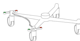
Castors \varnothing 125 central brake, at the sides (left, right or both sides)
